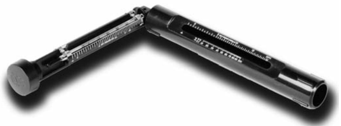
Figure 4. A photo of a sling psychrometer
